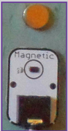
A magnetic sensor, which can detect positive and negative magnetic forces, with a magnet
