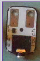
A touch sensor that functions like a MaKey MaKey connection, allowing a student to attach any conductive object with alligator clips, and make it a button
